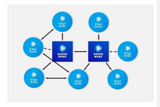
The edge nodes send a request to the supernodes, which registers, their MAC address and sends an IP lease confirmation to set an IP on the edge. The process is similar to DHCP. Thereafter the edges have layer 2 peer-to-peer communications directly with other edge nodes
